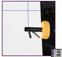
Diagram 2 Make sure that the face of the gauge remains in contact with the edge of the board as you draw the line.
